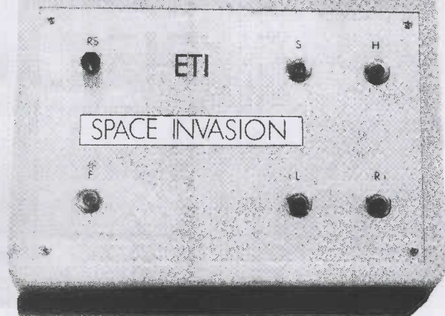
The face of the Space Invasion. The simple controls are reset, start (play), hold, fire, left and right.
