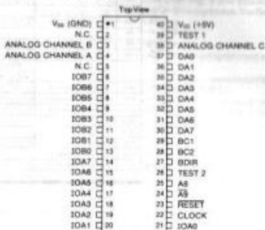
Fig. 4 AY-3-8910 PIN ASSIGNMENTS
