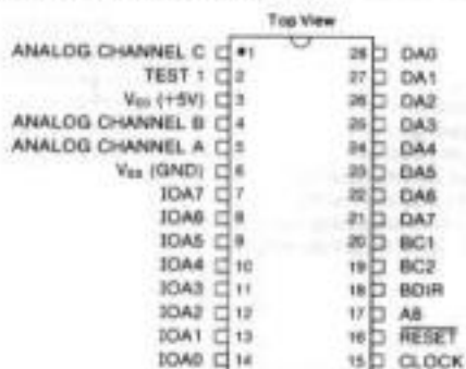
Fig. 5 AY-3-8912 PIN ASSIGNMENTS
