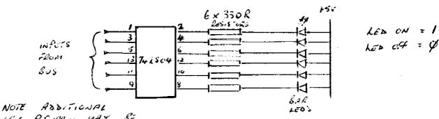
ASV P. SUPPLY MAY BE REQUIRED IF ALL 30 SECTIONS ARE USED - TYPICAL I = '700 MA
